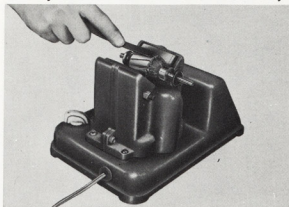
Fig.16-15 Armature Coil W5786 Short Circuit Test
