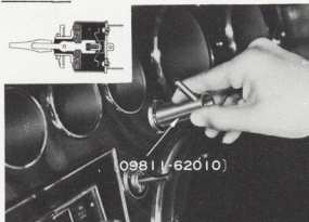
Fig.15-8 Removing Toggle V1514 Switch G0432
