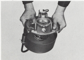
Fig. 13-32 Disassembling Booster V1792
