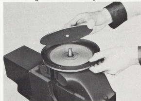
Fig. 13-43 Assembling V1797 Power Piston
