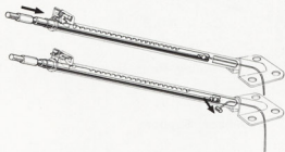
Fig.13-21 Disconnection of X6222 Cable No.1
