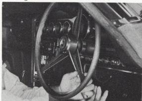
Fig.12-4 Removing Horn Button Stopper Ring V1297
