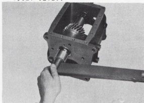
Fig. 9-17 Tightening Counter V1289 Shaft Front Bearing
