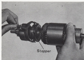
Fig. 7-19 Assembling Pinion W8642 Drive Lever
