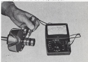
Fig.7-28 Testing Rotor Coil V2196 for Open and Short Circuits
